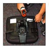
Remove the old mech, and replace with the new mech, positioning it over the four T-nut receptacles in the seat. Replace the bolts one at a time, with washer/spacers as before, and tighten them in rotation until all are secure.
