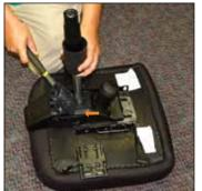
Next, firmly holding the cylinder with one hand, and strike the mechanism around the cylinder entry point with the hammer. Several strong blows may be required to dislodge the cylinder from mechanism. \*\*
