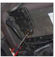
2. Locate the arm bracket where arm attaches to the seat. Locate the large Phillips head screw at the end of the arm steel, and remove it, setting it aside for later reinstallation on new armrest.
