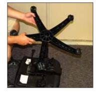
Reinstall cylinder, base and armrests using reverse of steps used to remove them.
