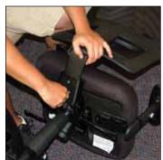
With screws started by hand, tighten all with the Allen-wrench to secure the back assembly to the mechanism.
