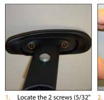
Locate the 2 screws (5/32" Allen-head) that secure the urethane arm pad to the arm support. You may find it easier to access by removing the entire arm support (Reference to *Arm Replacement* sheet). Remove the 2 screws, set them aside for later reinstallation, and remove the pad.
